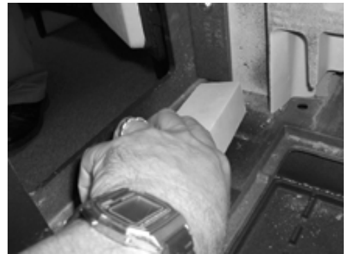
FIG. 6 Remove Lower Load Door Refractory
